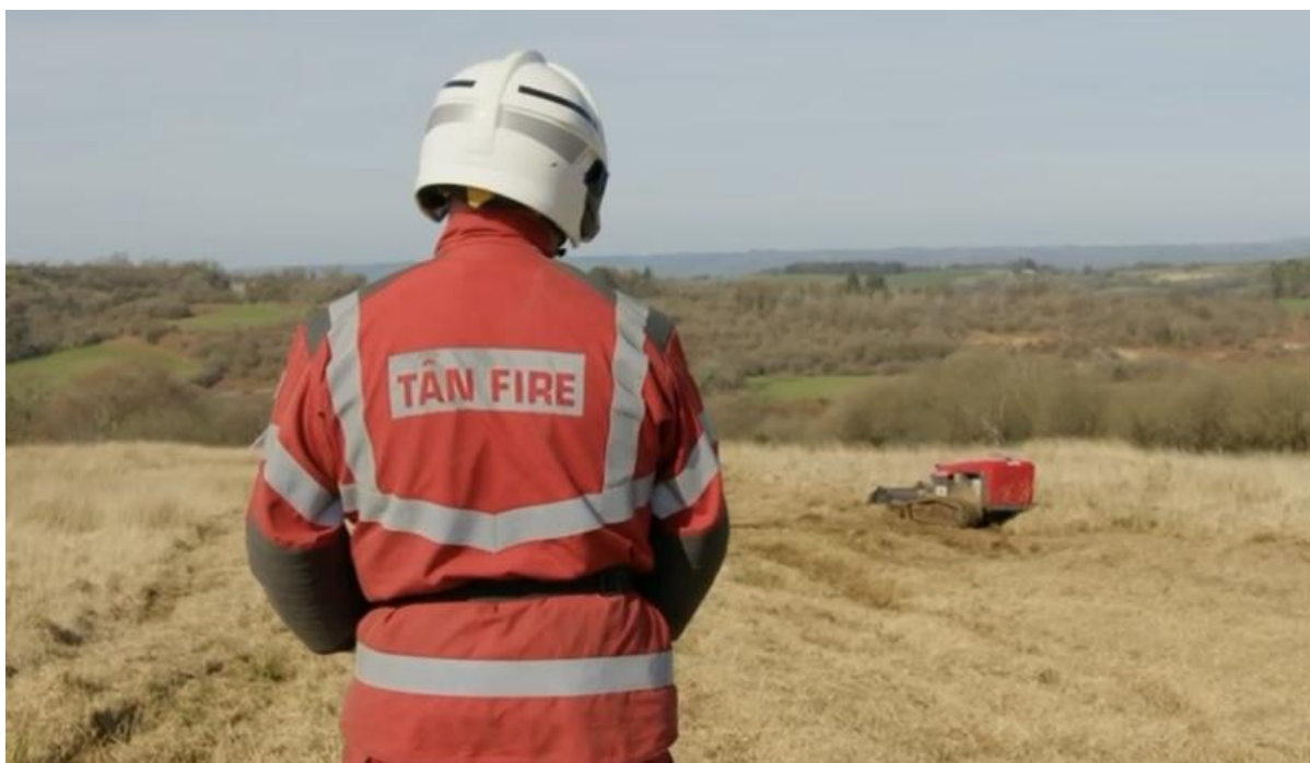
Plate 7: Firefighter cutting fire breaks using a robo-flail, Carmarthenshire. Photo credit Laurence Whitaker.
